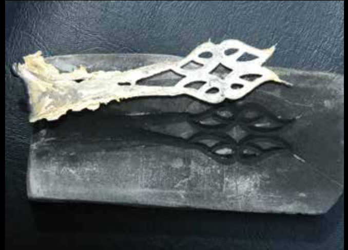
One of Dan Simplicio's tufa molds with casting poured by his son Dan Jr. It has an unusually large sprue (the silver to the left) and shows little nipples left by the air channels. All that has to be cut off and requires a lot of file work to finish.
