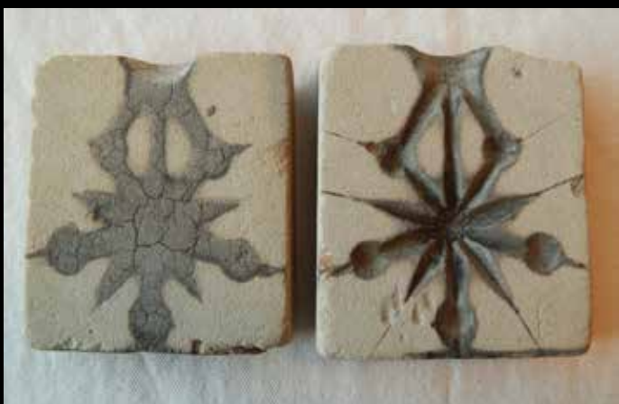
This is a rare tufa mold that still has its lid. This is a Stephen Gia piece but it is hard to figure out what the finished casting would look like—apparently a five pointed star.
